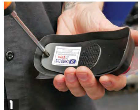
Using a #2 Philips screwdriver, Tony removes the backing cover of the inView light.
