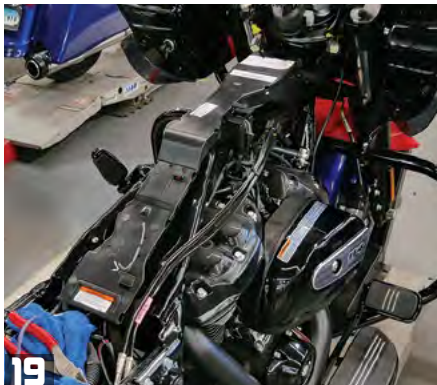
18 He wraps all the wires in black tape and runs it down the backbone of the frame, alongside all these other wires.
