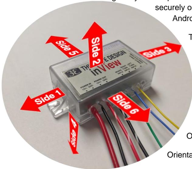
The motorcycle unit must be installed such that one of the 6 orientations below is facing the direction of travel. For example, if you select Side 2 below, the side with the **inView** sticker faces toward the front of the bike. It needs to face directly forward. Any tilt or deviation other than directly forward will diminish the functionality of passive braking.
